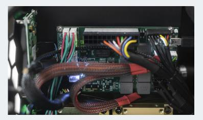
The Controller Board serves as the central intelligence of the entire system, acting as its brain. It plays a pivotal role in orchestrating the seamless operation of various components. All sensors, fans, pumps, the display, and the motherboard are intricately linked to this vital hub.
